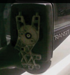
MISSING MIRROR COVER
